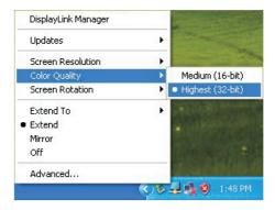
• **Screen Rotation:** This item allows you to rotate the screen by 90, 180 or 270 degrees, on the additional monitor.
